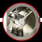
Three blade stainless steel mixer with interchangeable scrapers
