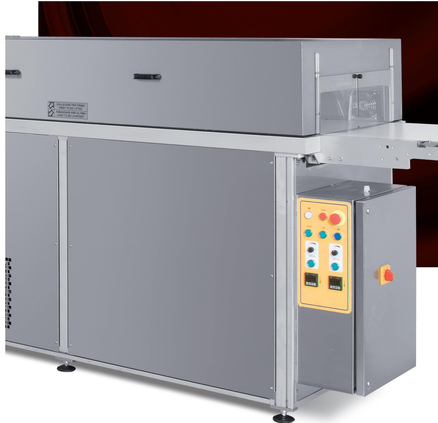
**GB-** Used to obtain a perfect drying of enrobed products. The cooling process is performed by a cooled air loop controlled by a thermo-regulator. A low power cooling unit controls humidity in order to obtain an excellent final result. The belt feed speed is adjustable. The tunnels are available in different lengths and widths, according to the user's needs. An independent and thermo-regulated cooling unit is placed every 6 metres along the tunnel, so that different temperatures can be set.
