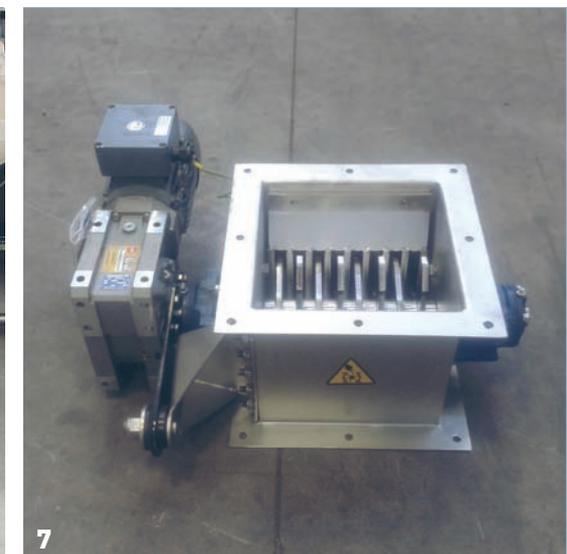
1 Dump stations with minisilos 2 Diaphragm valve 3 Antidust filter 4 Dump station with lump breaker for sugar 5 Vibrating cone 6 Dump station with silsystem 7 Lump breaker
