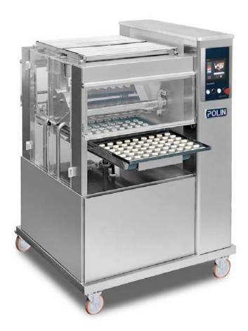
Multi-purpose depositor that can be used for either single or dual color dough processing. Four rollers built-in head, controlled by PLC allows for a large range of single or dual color cookies production. It is also possible to produce filled or topped products. Two doughs can be deposited at once, or filling can be done inside the encrusted cookies.
