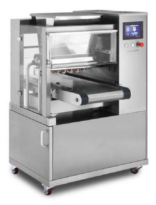
Multi-purpose depositor machine. The 100 program computer and design allows the operator to process a wide range of doughs and batters into many types of final products
