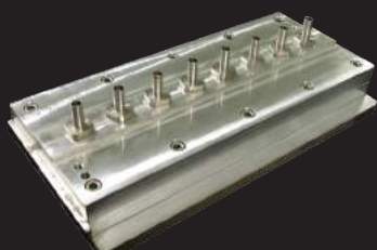
Dosing head for pralines This dosing head is made based on the dimensions of the mould
