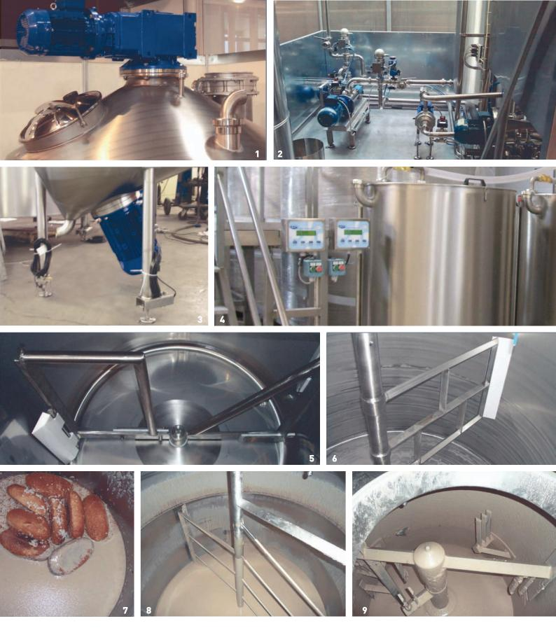
1 Agitator 2 Metering pump 3 Inclined extraction in dissolver 4 Tank weight control by WP 5, 6, 8, 9 Scraper (details) 7 Bread re-work in liquid form
